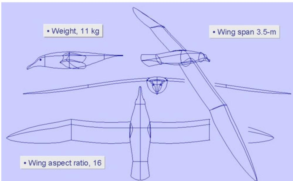
weighs 11 kg, or 24-lb. Its 3.5-m wing has an aspect ratio of 16. As we shall see, high aspect ratio is essential to reduce drag during high-g turns associated with dynamic soaring.
